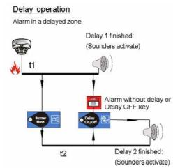
The activation mode of sounders can be configured by zone, with or without delay for manual call points or detectors. Sounders may also not be activated by a specific zone.
