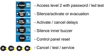
\*2 In Access level 3, the push-buttons have selection functions.
